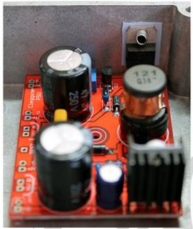
PSU: Keep a safe gap (2-3mm) between PSU pcb and enclosure, I used 2 strip thick of double sided tape to secure it. But you could also use a standoff.
