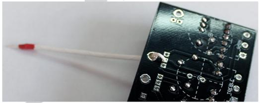
Pull back the cable, insert the hot in it's pad, make sure the shield sits nicely in the shield pad. From the solder side of the PCB, simply put your iron in the gap between shield pad and braided wire and flow the solder in. Don't worry about the shield melting it won't. Hot is soldered on the component side, so flip that biatch over!
