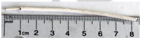
Hot End: Cut the braided shield so it is flush with the outer sleeve.
