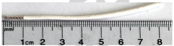
Hot End: Strip 1cm from the outer sleeve. The Telflon sleeve is very durable and slippery when stripping, you can pull off the sleeve if you're not careful.
