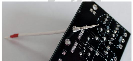
Installation: From component side of PCB; push the cable through the shield hole further than it needs, to give a smooth rounded shape to the Hot core.
