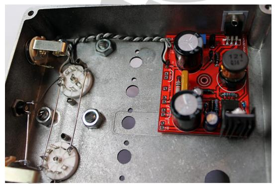
Heater, Ground & 9V wiring: Connect as above. You can twist these for neatness should you feel so inclined. Heater goes to the bottom rail. Ground to the top and 9V to the power jack.
