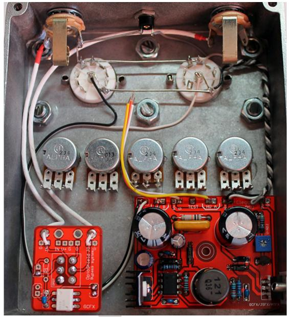
Install your OptoShield bypass system. Approximately 13cm of shielded cable for the input, and 20cm for the output.
