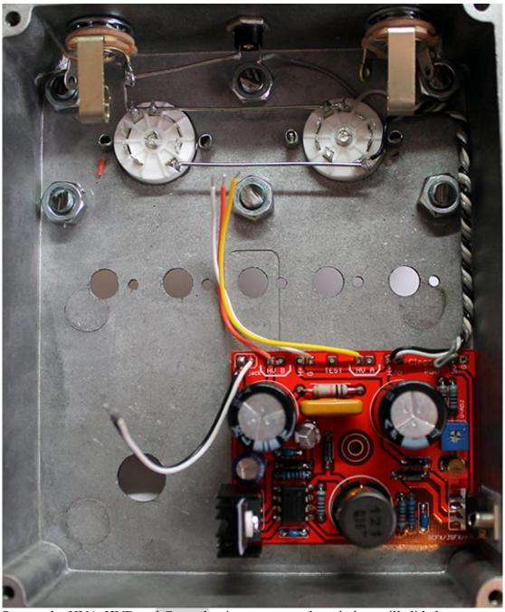
Pre cut the HVA-HVB and Ground going to preamp board, they will slide between two pots. Also prepare the wires to hook the OptoShield.
