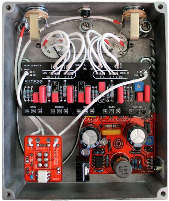
Solder wire and cable from pin8 to pin1 for V2, you will likely want to solder Pin2 before Pin1, goes better
