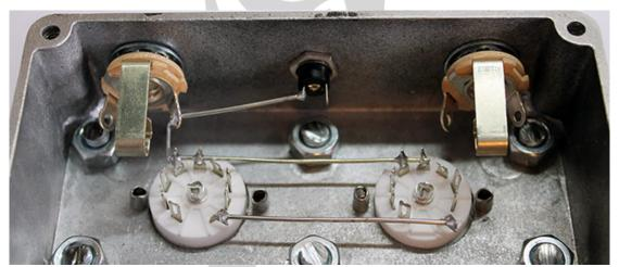
DC Input Ground: Connect DC jack negative tab to input jack sleeve then to the ground rail.
