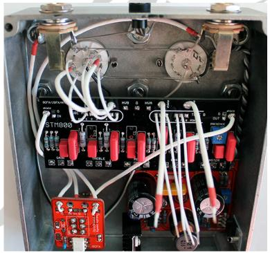
Solder wire and cable going from Pin1 up to Pin8 for V1
