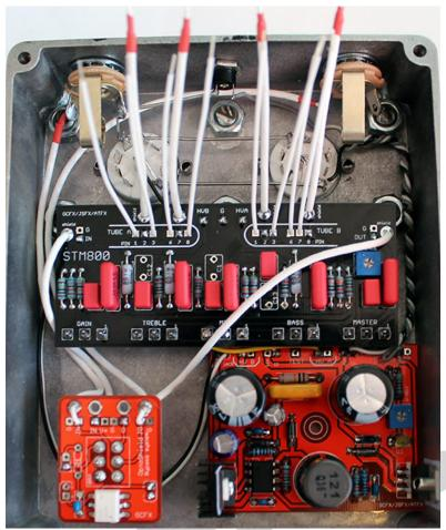
Connect the preamp in and out cables on the Opto so they're out of your way.
