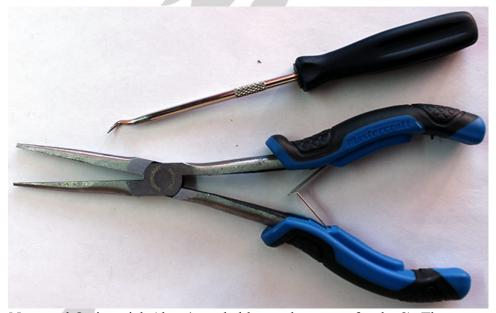
Long Nose and O-ring pick (there's probably another name for that?). These come very handy in this build, the longer and finer reach of the pliers is much appreciated and the O-ring tool is very handy to re-route wires in tight places. You should be able to find that tool for cheap in any automotive parts store, usually comes in a kit of 3, straight, 90degree and angled. Note from Juan: I use tweezers for this sort of thing.
