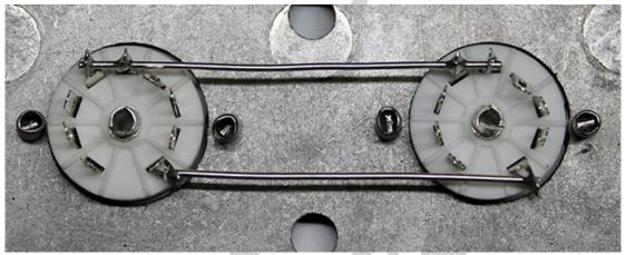
Heater & Ground Rails: Using Bus wire for a neater install, twist and bend tube socket tabs so they align and don't short with the other, work them gently but firmly. Like you would a woman.
