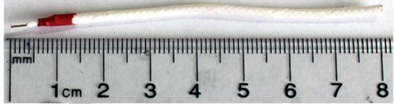
Hot End: Cut a 1cm piece of heat shrink tubing. Put it half & half on the core sleeve and outer sleeve and shrink it in place. The hot end is now complete.
