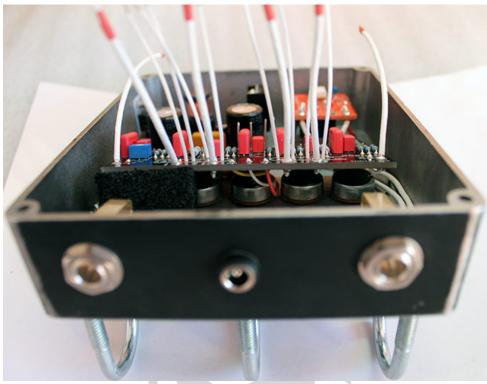
Install preamp on pots, but don't solder that yet. Tilt up the tube side of PCB, put something under so it holds and don't pops it from the pots. I used a piece of IC foam that comes handy for many other thing in my building habits... Put HVA-HVB and Ground in their respective pads, using a little color coding with the wires here, comes in handy
