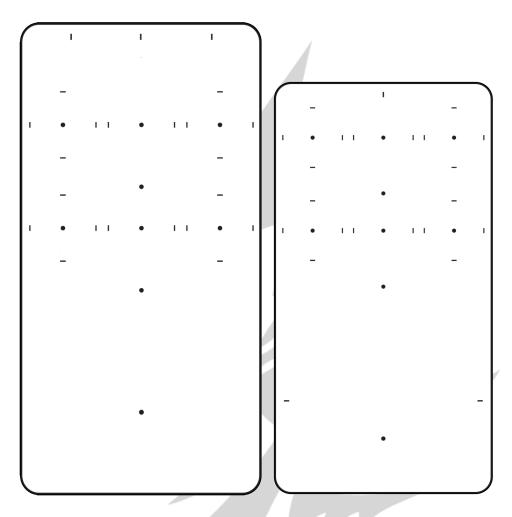
The PCB was designed to work either in a1590B or 125B enclosure. There are extra ground pads and 9V pads to give alternate ways of wiring it up, they don't need to be all connected. Also, if a bypass daughter board with LED is used, you can omit the on-board current limiting resistor (CLR).
